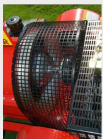
The enclosed turbine air intake provides minimal intrusion of debris in the turbine chamber.
