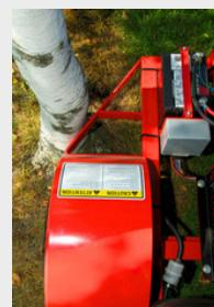
The fenders are constructed of steel with exclusive impact resistant bumpers to reinforce the overall structure.
