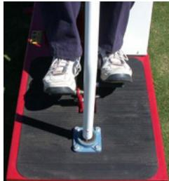
Smooth Roll has many features that make it simple and easy to operate. Feathertouch foot-operated directional controls make Smooth Roll simple and safe. Alternative pedals are used for braking. Simple steering controls enable a **Z-Pattern movement** producing a double roll every time.
