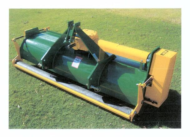
2. With the TT Renovator on the ground, measure the PTO shafts required length (allowing enough adjustment for the machine to be lifted).
