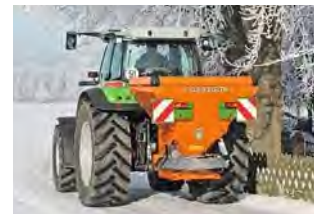
E+S winter service spreader, 300–1,000 l hopper capacity
