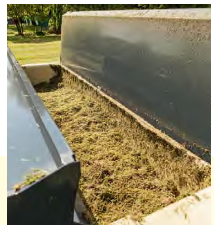
⊕ Compacted, cut material in the collection hopper
