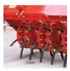
Six heads containing two wheels float independently to follow your most demanding contours. Weight trays are standard to aid penetration on compacted areas.
