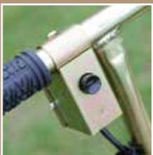
Simple on-off 'push-button' for instant control of paint delivery, and benefits with having the battery charging socket on the rear of the switch housing.
