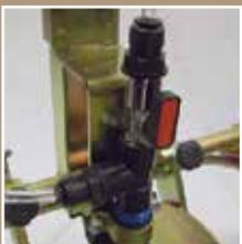
The prime valve is located at the front of the machine for ease of use, and protection from accidental damage. The system allows for priming direct onto the line to avoid paint spillage on the field.
