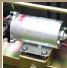
The heavy duty diaphragm pump, delivers consistent pressure, for high quality line-marking.
