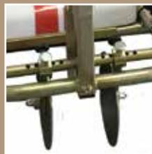
Pre-drilled disc spacers for quick, line width changes, and front bumper bar that protects the nozzle assembly from accidental damage during transit.
