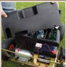
Removable cover provides protection and allows easy access to the electrics, pump and battery. The cover is manufactured from precision moulded MDPE.
